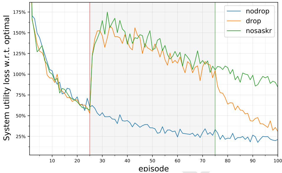
Figure 9.6: System utility comparison to the system optimal in the volatile system, as measured by the percentage difference in utility between the specified algorithms and the <nodrop> baseline algorithm.
